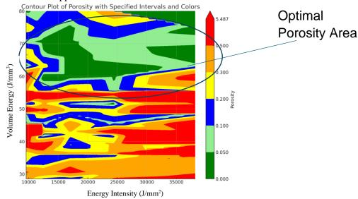
Figure 1 - Contour plot of porosity as a function of energy intensity (J/mm<sup>2</sup>) and volume energy (J/mm3) during L-PBF processing of pure iron.
